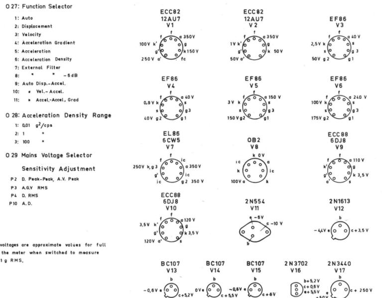
The enclosed voltages are approximate values for full deflection on the meter when switched to measure acceleration 1g RMS.
