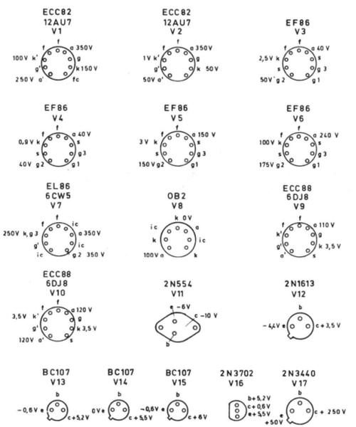
The encircled voltages are approximate values for full deflection on the meter when switched to measure acceleration 1g RMS.
